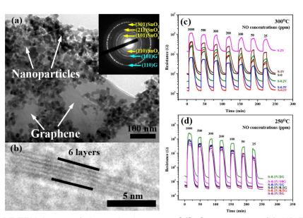
**RESULTS:** (a) BF-TEM image of the optimal  $0.5 \text{ wt}\%\text{G/SnO}_2$  composite, (b) HR-TEM images of multilayer graphene (G), change in resistance under exposure to NO (25-1,000 ppm) of (c) undoped SnO<sub>2</sub> and 0.1-2 wt%V-doped SnO<sub>2</sub> at the optimal working temperature of 300°C and (d) 0.1-10 wt%G/0.1 wt%V-SnO<sub>2</sub> sensors at the optimal working temperature of 250°C.
